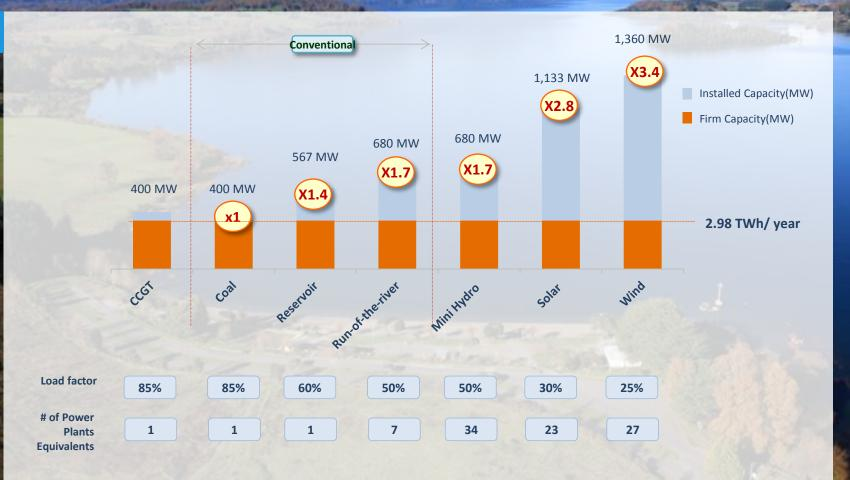
(1) Considers: CCGT= 400 MW, Coal= 350 MW, Hydro - reservoir= 400 MW, Hydro Run-of-the-river= 100 MW, Mini Hydro = 20 MW, Solar= 50 MW, Eolic = 50 MW
